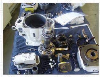
Overhaul of hydraulic component (e.g. Motor, pump, and cylinder)
