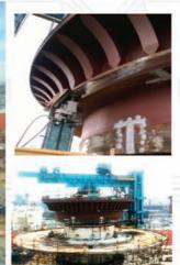
On-site Machining of Turret Shaft and Caisson
