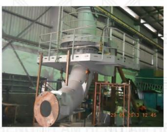
**Fabrication and Casting of Swivel Bend**
