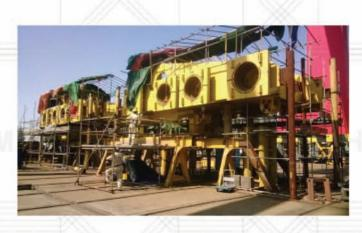
On-site Milling and Boring of Traveling Cradle
