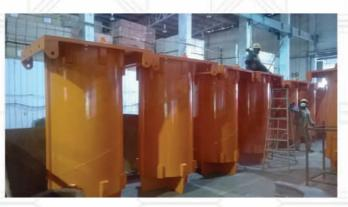
**Fabrication of Piling Sleeve and Support Beam** Clamp
