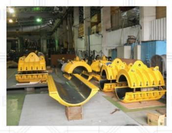
**Fabrication of Lifting Clamp and Anchor** Clamp
