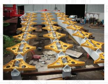
**Complete Fabrication of Offshore Drilling Equipment (Riser Fingerboard) with Installation and Hook-Up Service**
