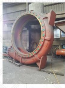
**Casting for Pump Casing**
